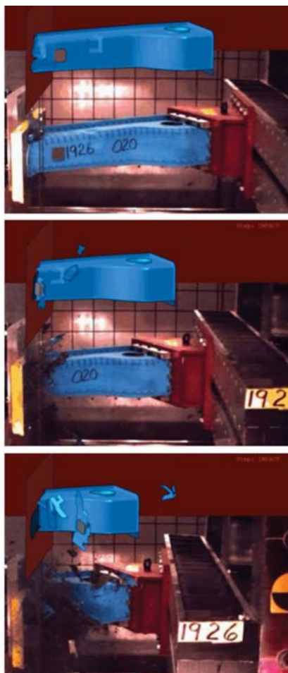
Fig. 3: The rail crush example is run in CZone for Abaqus, which is an add-on product to Abaqus/Explicit. Image courtesy of Engenuity, Ltd.
