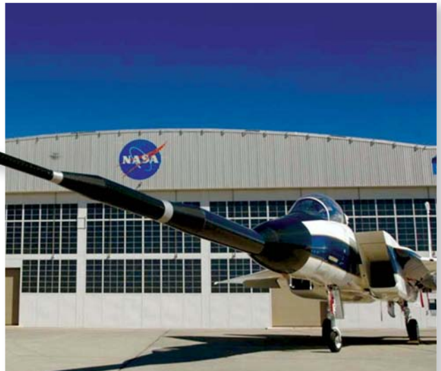
Fig. 1: In 2006, Gulfstream partnered with NASA to test their "Quiet Spike." The thought was to push the shockwave far out in front of the plane.
