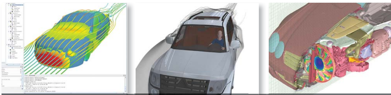
Fig. 4, 5 and 6: Examples of what can be done with software. You transfer results such as the pressure fluctuations to a structural software, such as Simulia's Abaqus, NASTRAN or acoustic software such as ACTRAN, for further analysis, such as noise predictions inside the cabin of a car. Images courtesy CD-adapco.
