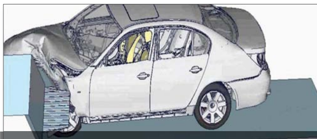
Fig. 1 and 2: The crash management system is designed and maintained during the crash scenario, including the crumple zone areas in the front and rear. Images courtesy of BMW.
